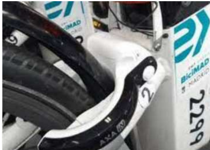
Figure 13: View of the new locks installed at BiciMAD e-bikes to allow freefloating operation
