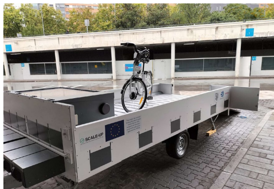
Figure 11: Other detail of the docking positions of the mobile BiciMAD station, once the docks are removed when the mobile station needs to be moved
