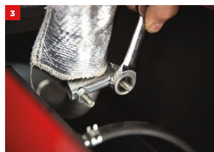
3) Remove lower exhaust clamp to release the silencer from the engine
