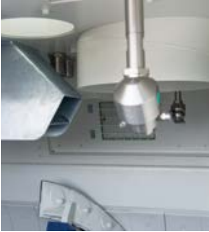
A total of four motorised cleaning jets ensure the mixer looks as good as new at the end of the working day. On the left in the photo: water is distributed over the entire width of the mixer.
