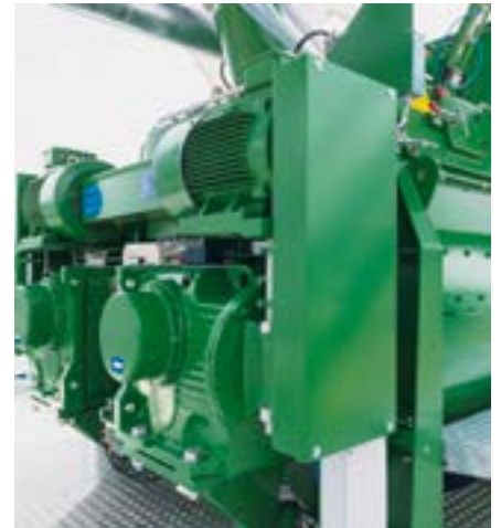
The twin-shaft compulsory mixer features two synchronised motors and two gear systems connected by toothed belts with protection against damage.
