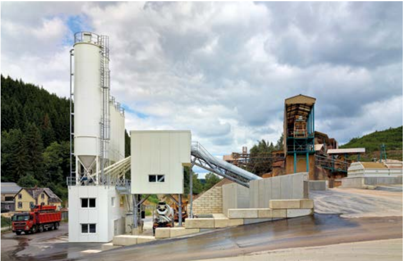
The Ammann Elba concrete mixing plants can be equipped with winter cladding as an option, like on this CBS 180 TB Elba.
