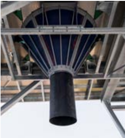
Lowerable mixer discharge funnel clad with EWP wear protection.
