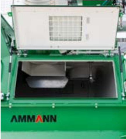
Generously dimensioned maintenance doors facilitate maintenance and cleaning work.
