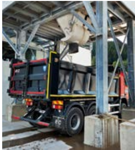
The CBS 130 TL Elba on concrete foundations. The plant can also be supplied on steel frame foundations as an optional extra.
