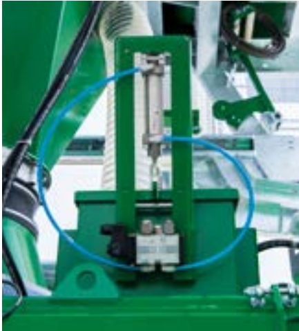
Quality control via camera system: mounted to a pneumatically operated camera shaft directly on the mixer.
