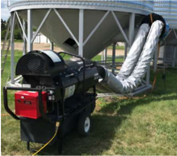
Figure 4-9. Direct fired heater ducted to bin aeration inlet (upstream).
