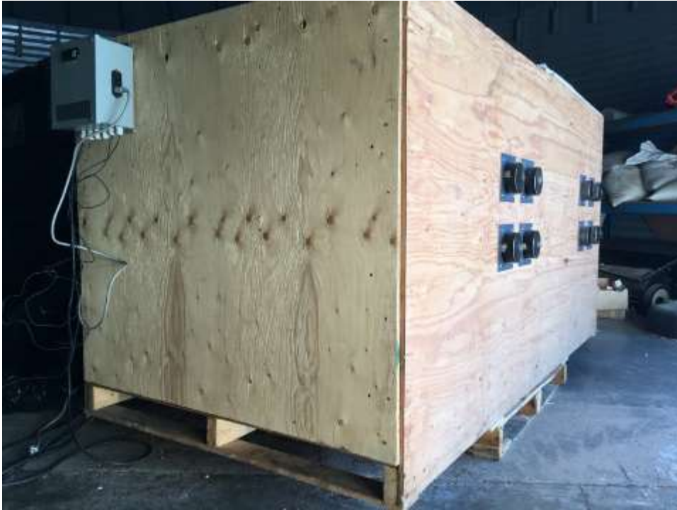
Figure 3-9. Preheated chamber used to supply heated air to bins.
