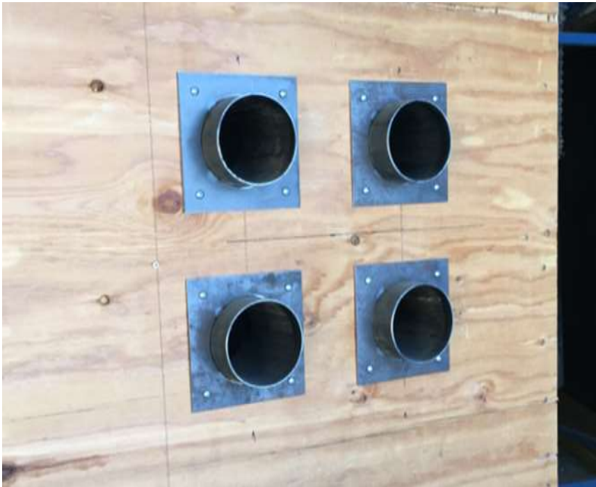
Figure 3-11. Intake vent holes located on the side of the preheat chamber.
