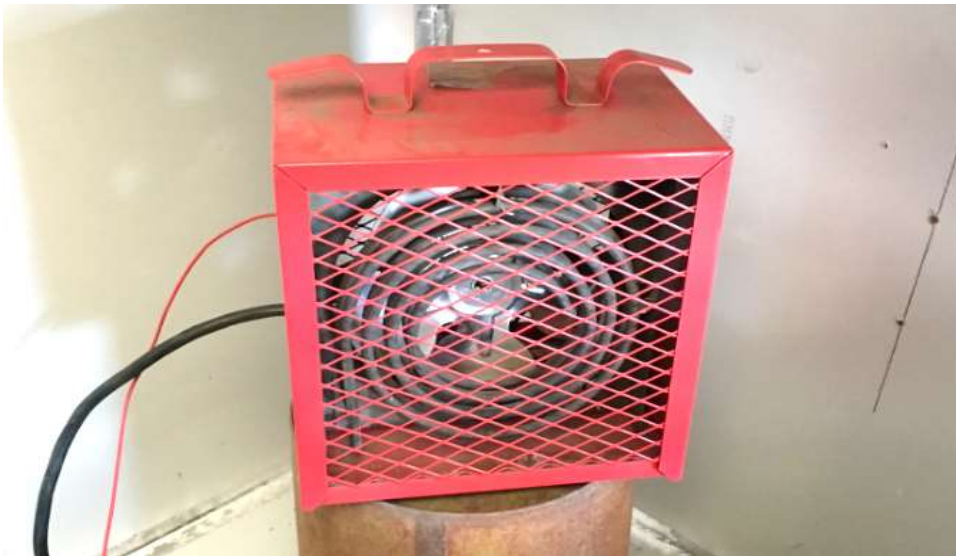
Figure 3-10. Electric heater located inside preheated chamber.
