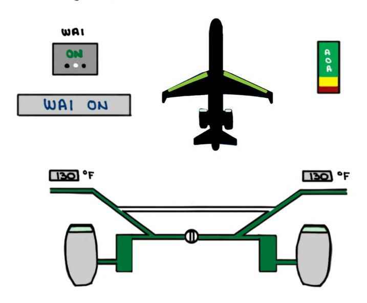
Wing Temperature <u>must be</u> > 100°F and aircraft altitude > 1,500° AGL for the control Law logic To change
