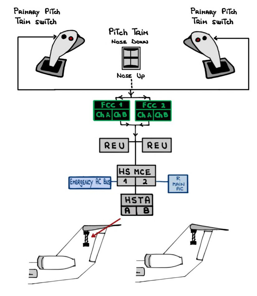
In the event of loss of communication from the FCCs The sidestick pitch tain switches won't be available. The pedestal switch bypasses the FCCs and signals the HS MCE. The stab moves at a constant rate
