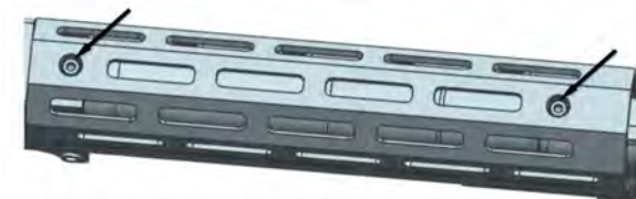
Fig. 17 Removing the two M4x8 hex socket head screws
