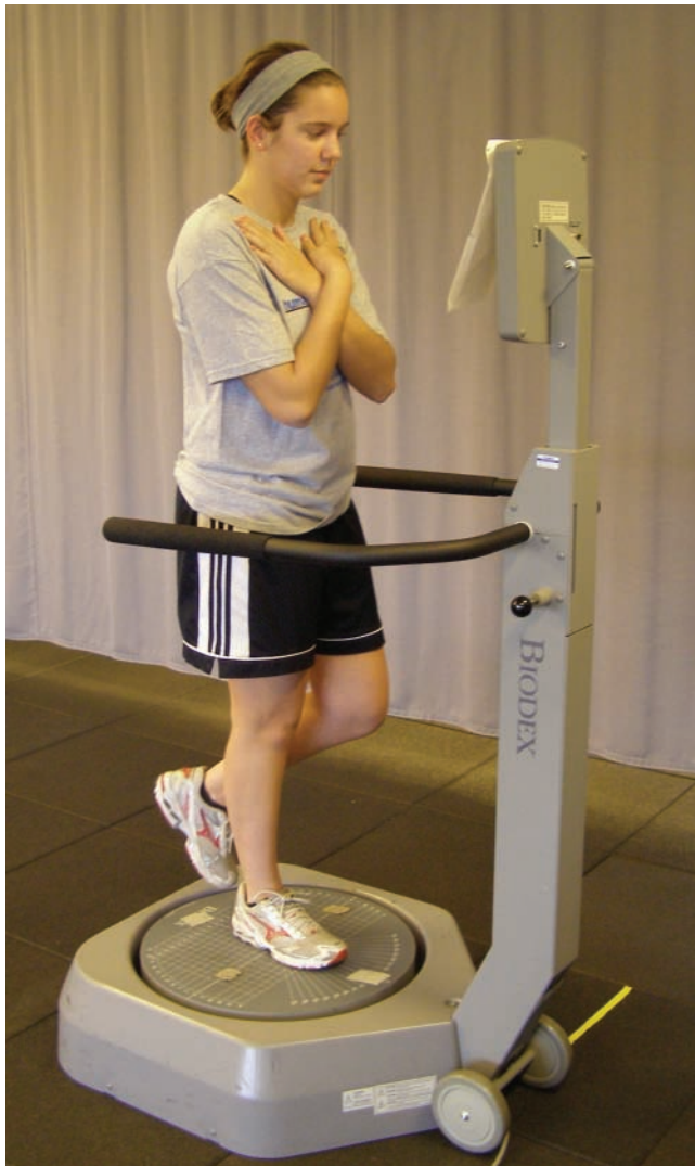
Figure 3. Participant during the assessment of postural stability using the Biodex SD Stability System. The individual is in a unilateral stance position with the contralateral limb flexed and both arms crossed at the chest. The participant is tested with eyes open, but receives no visual feedback on performance during the testing session.
