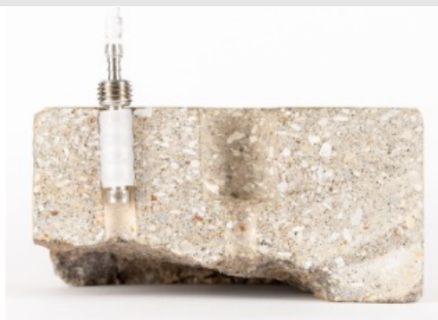
Subslab sample probe in foundation
