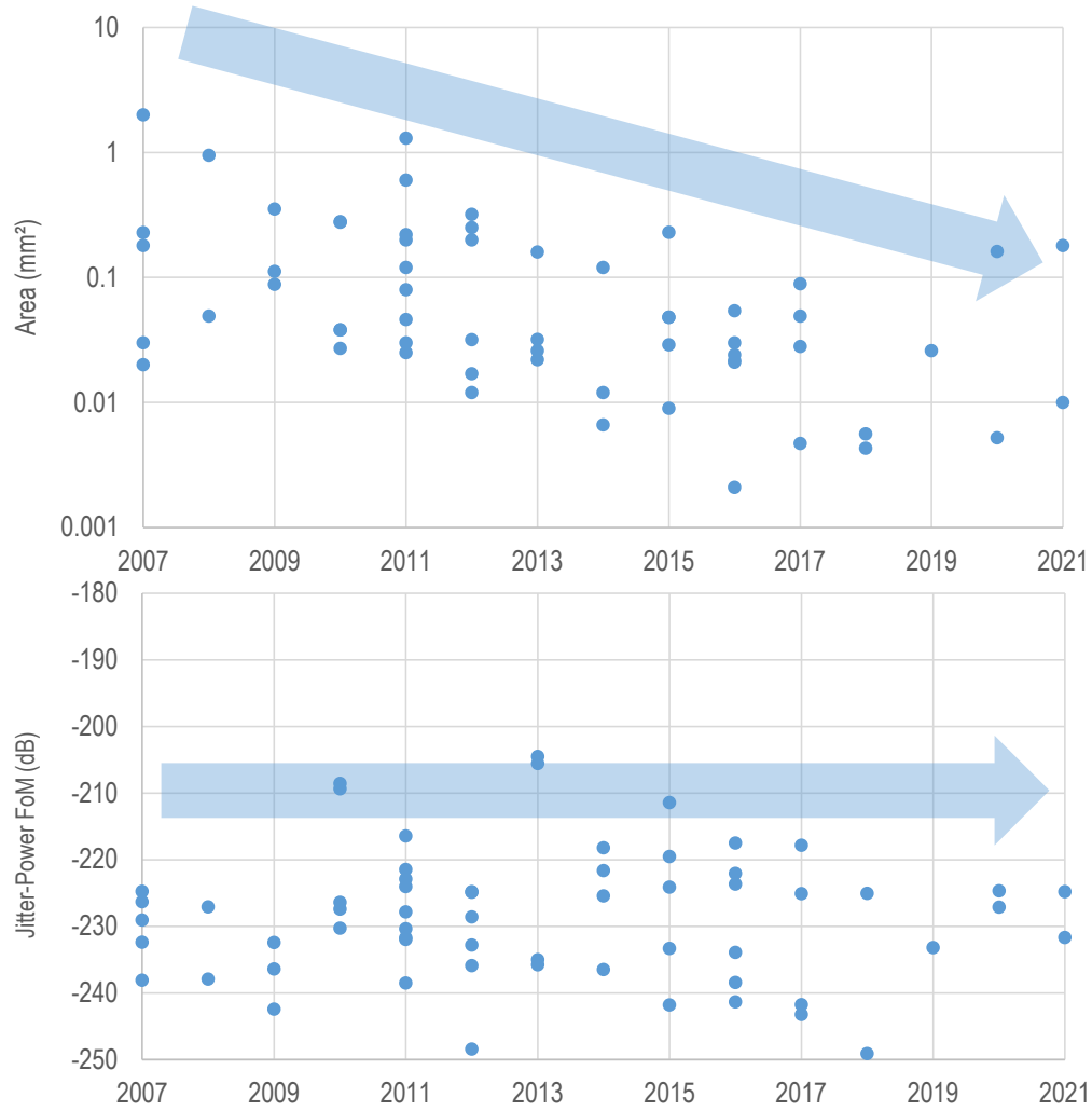
Figure 1. Digital phase-locked loop (PLL) and multiplying delay-locked loop (MDLL) trends in area and key figure of merit (FoM), defined as: \text{FoM} = 10 \times \log_{10}\{ (\text{Jitter}_{\text{RMS}}/1\text{s})^2 \times (\text{Power}/1\text{mW}) \}.
