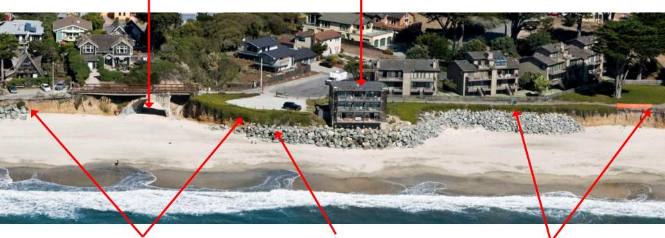
County proposes aluminum replacement bridge and armoring to wrap both sides of the mouth of the arroyo, connecting to existing shoreline riprap.
