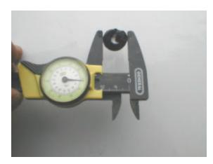
**Figure 3-19**. Dial caliper used to measure black turban snail shell sizes.
