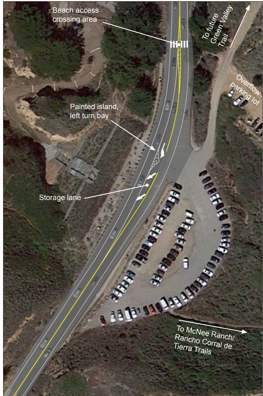
Improvements are shown above to help vehicles enter and exit the parking lot, reduce conflicts between turning vehicles and through traffic, and help pedestrians cross the highway.
