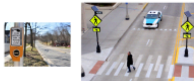
Push button activated rectangular rapid flashing beacons use an irregular flash pattern that is similar to emergency flashers and police vehicles to alert vehicular traffic.
