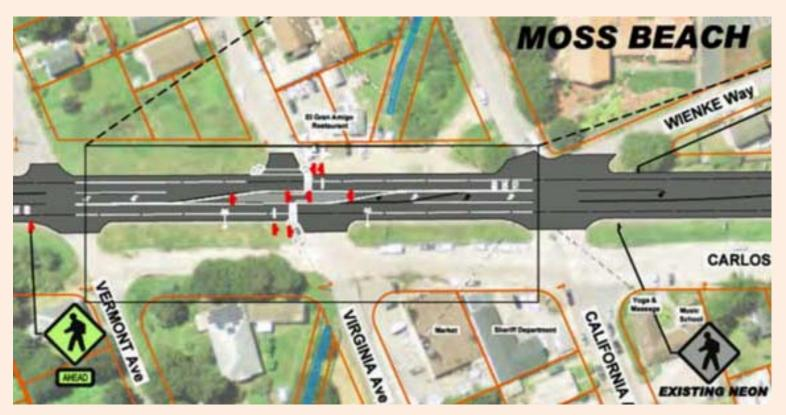
No pavement widening required for this project. Cross-highway traffic closed at Virginia – right turns OK.
