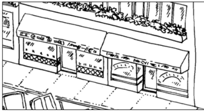
Figure 6: door and window canopies
