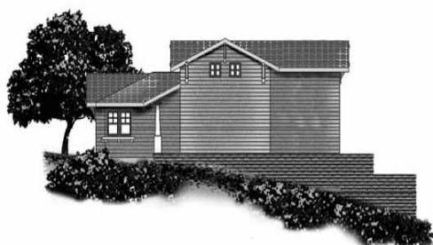
Structure is not suited to the terrain. Extensive grading was used to create building pad, and to terrace site beyond the immediate vicinity of the structure.
