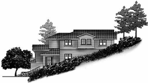
Building forms step down with the existing grade and there is no unused under-floor space.
