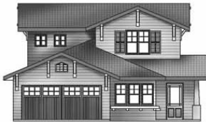
This second story addition centered over the lower floor away from property lines appears less boxy.
