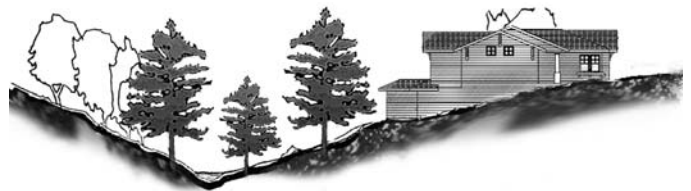
Structure is set back to avoid alteration of natural drainage feature.
