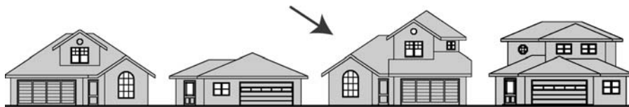
The revised design became compatible with its neighbors by stepping back the second story and providing variation in the roof and building forms.
