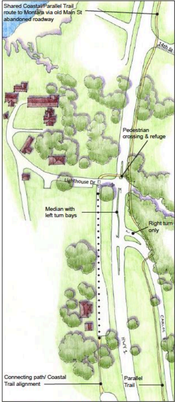
The addition of medians, left turn bays, trails and designated crossing to connect trails on opposite sides of the highway is shown above.
