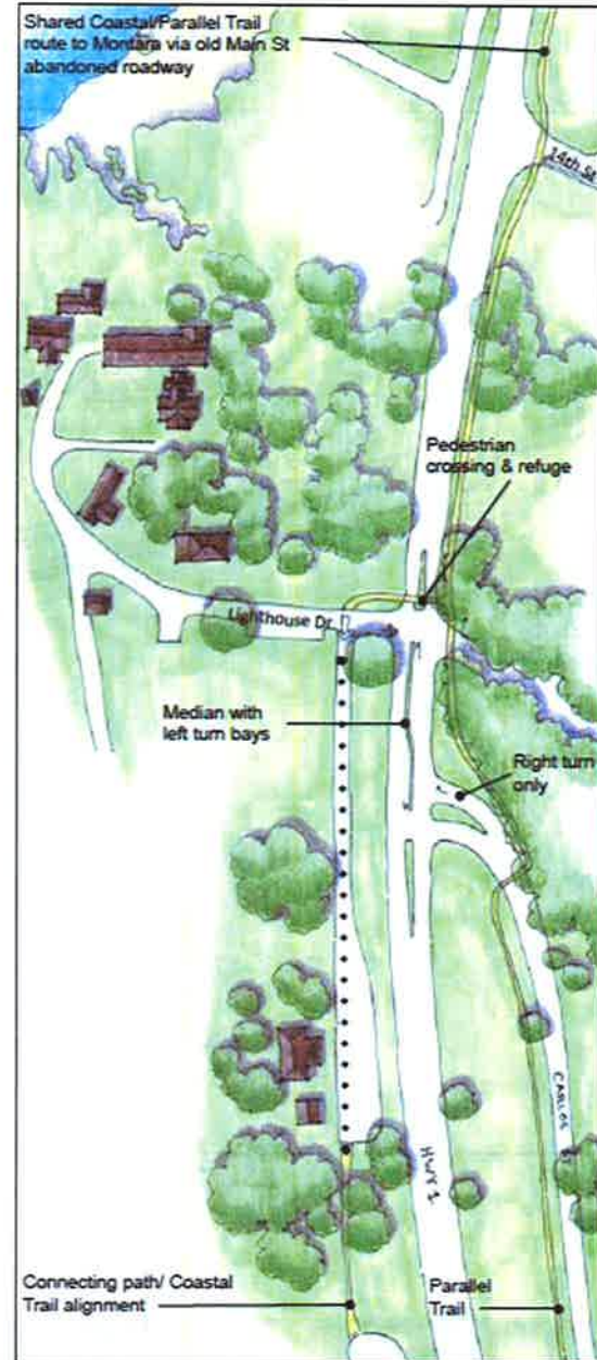
The addition of medians, left turn bays, trails and designated crossing to connect trails on opposite sides of the highway is shown above.
