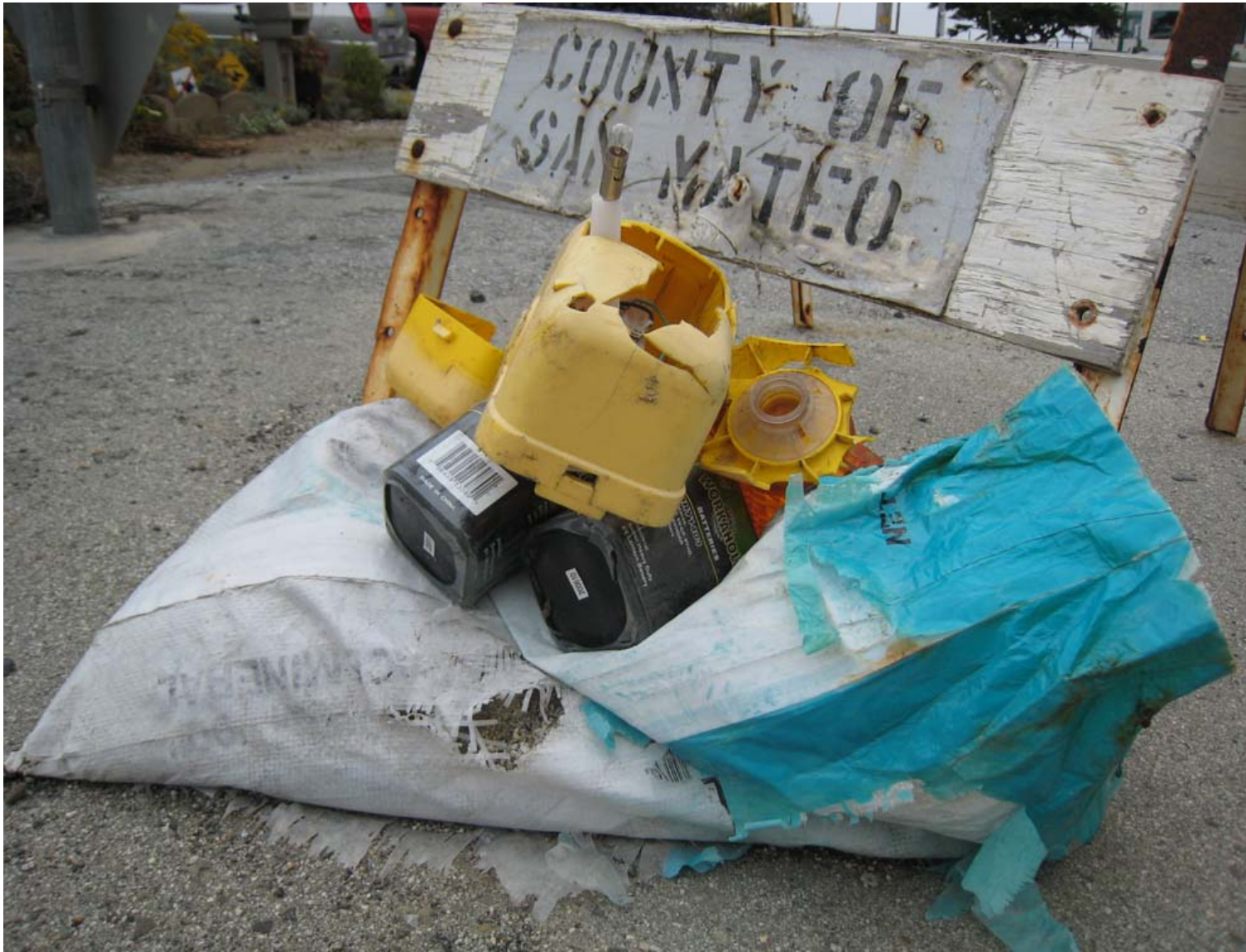
Plastic sand bags on Ocean Blvd in Moss Beach, degraded within one year, with pieces flaking off and blowing/washing their toxins into the ocean.
