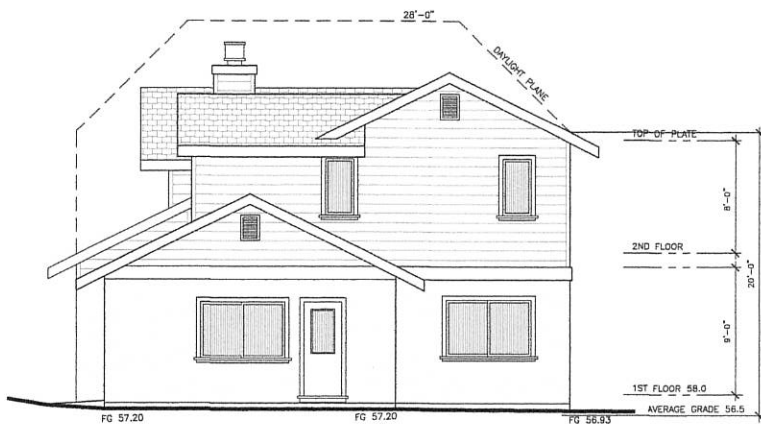
④ NORTH ELEVATION SCALE: 1/4" = 1'-0" (FRONT)
