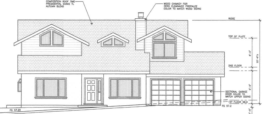
① EAST ELEVATION SCALE: 1/4" = 1'-0" (FRONT)
