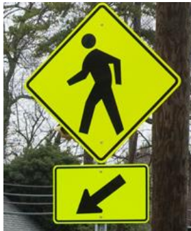
Figure 6: Typical Pedestrian Crossing Signage (W11-2 & W16-7P)
