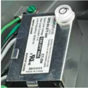
Internal Bubble Level facilitates installation
