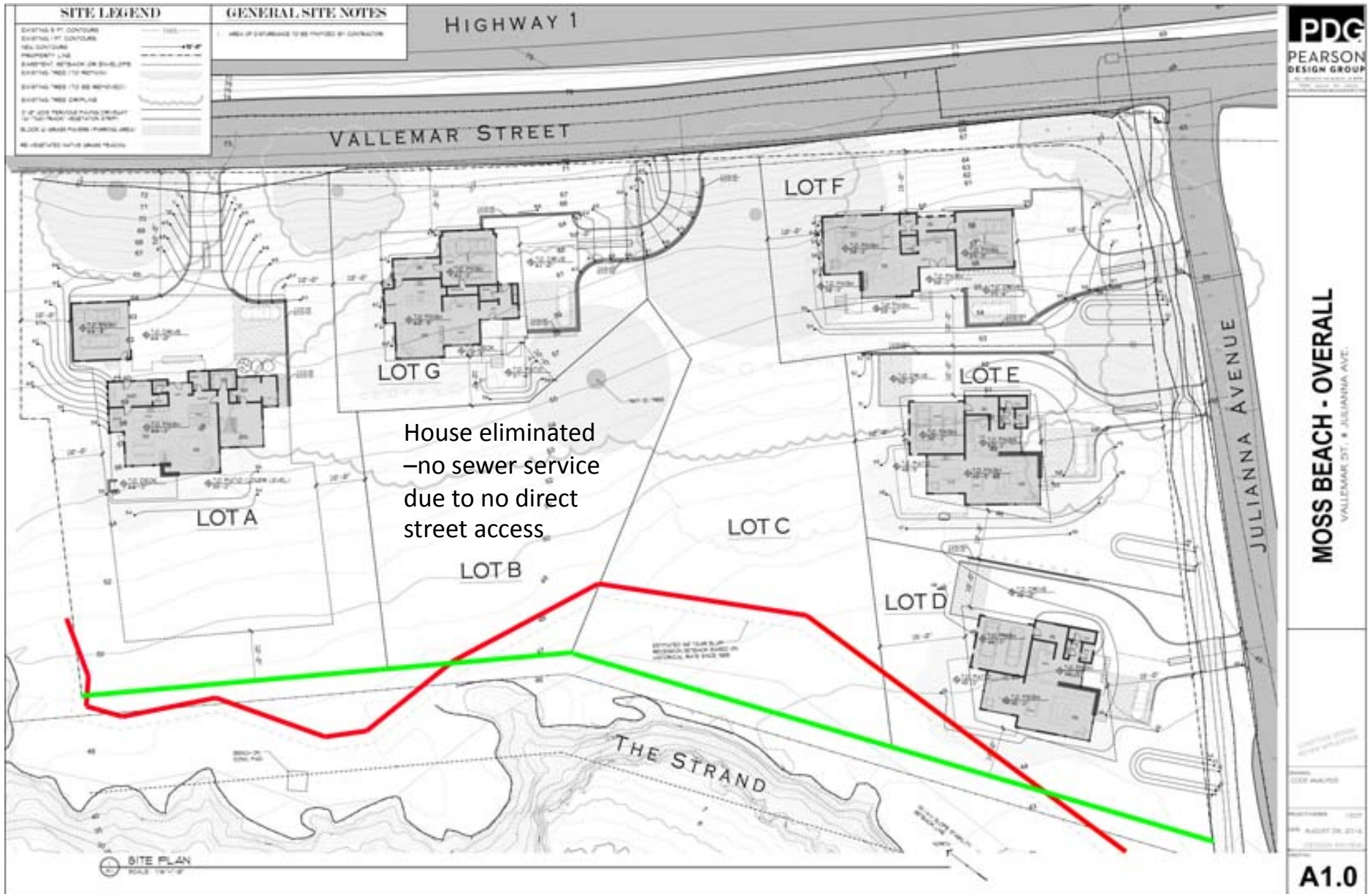
5-house site plan – Aug 2016 Red = estimated 50-year bluff retreat (per HKA) Green = property line
