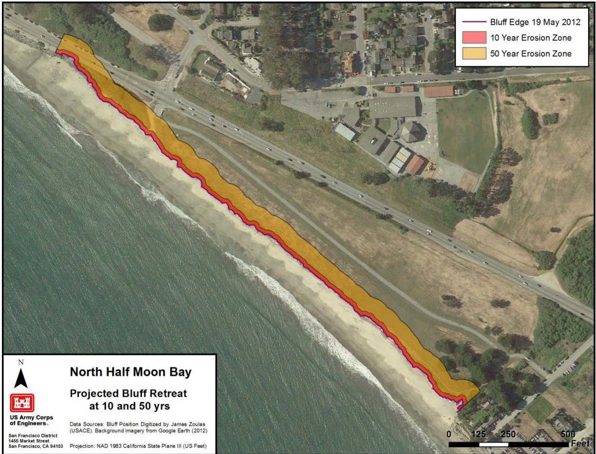
Figure 74: Extent of projected bluff retreat at 10 and 50 years, based on the estimated retreat rate of 1.64 ft (0.50 m) per year
