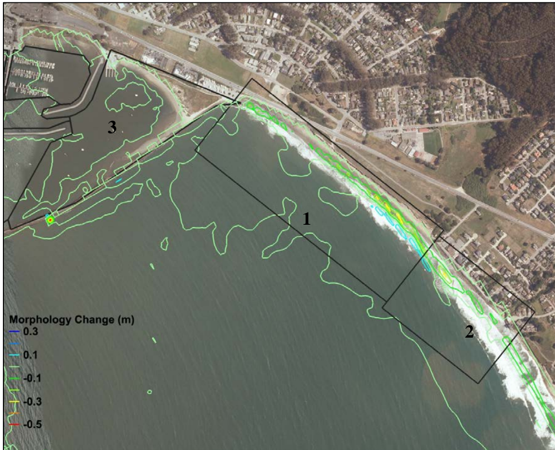
Figure 61. Erosion and accretion from June 2009 to November 2009 (6 months). The boxes outline the analyses areas
