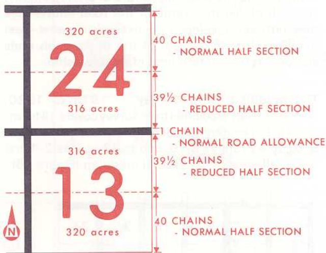
Figure 22 — A closer look at sections 13 and 24 of a typical township of Saskatchewan's modified third survey.
