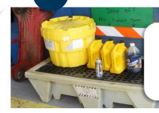
Always have secondary containment, like a spill pallet or doublewall tank.
