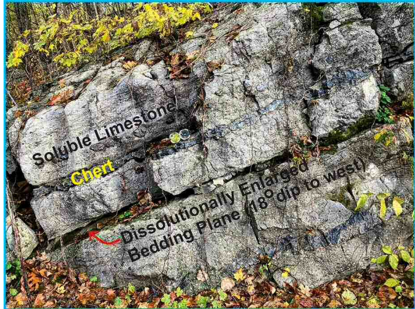
Figure 4. Steeply dipping Onondaga limestone along Hommelville Road. The Denier site is ~ 1,125 feet to the south where the bedrock dip is somewhat lower but still steeply dipping to the west.
