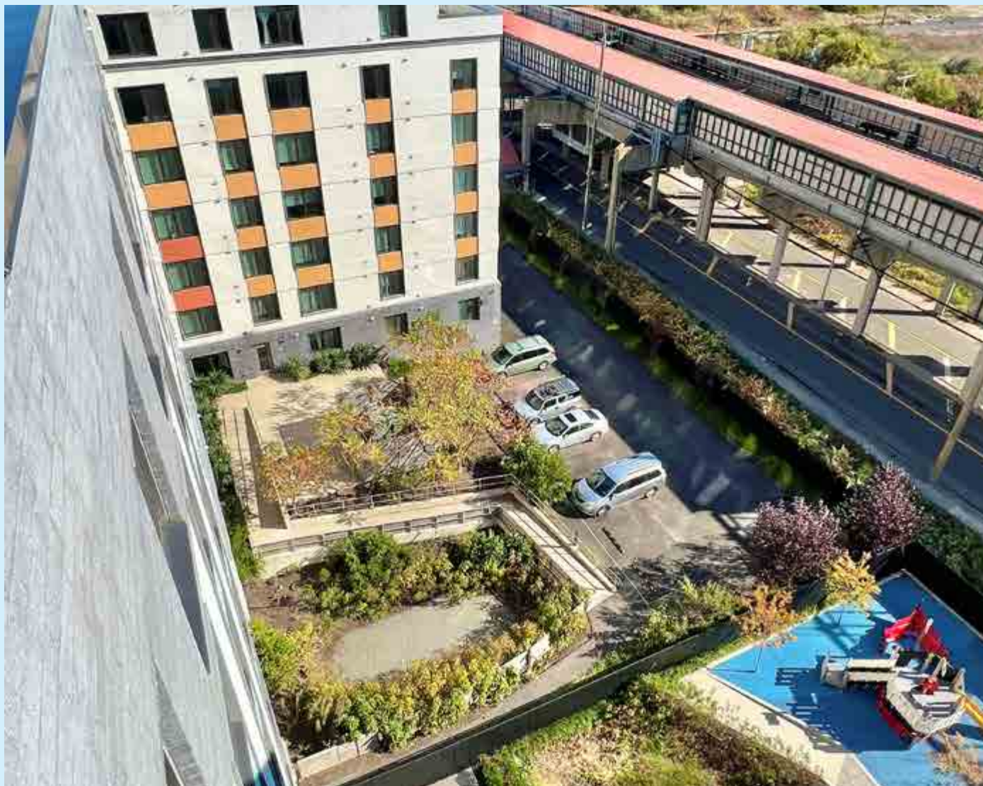
Wetland plantings, porous paving, and structural soil at Beach Green Dunes help to mitigate flooding by absorbing stormwater, and lowering groundwater. Credit: Local Office Landscape + Urban Design
