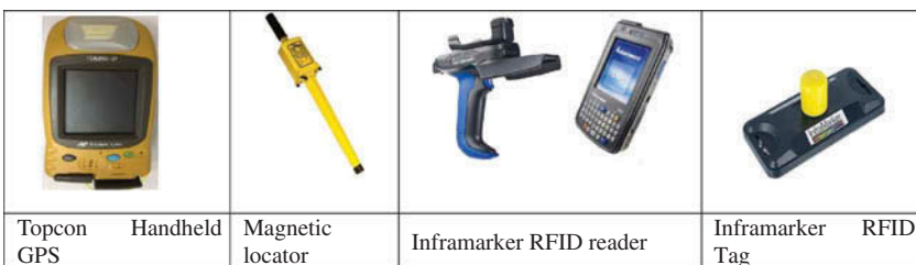
FIGURE 1 Technologies used for facility retrieval. GPS = global positioning system; RFID = radio frequency identification.
