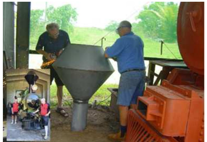
L_R Doug Benkendorff & Derek Marshall making the new stack for the KRAUSS Loco
