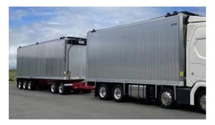
There are a variety of bin designs, which are suitable for grape cartage. All bins must meet food grade standards by either being alloy, stainless or covered in a food grade paint. All sealants and grease must be food grade. The length, height and load capacity of the bin will determine the requirements for baffles and splash backs. Splashback and baffle technical designs will be left for the operator to determine.
