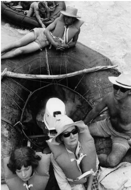
Rob Elliott hanging out on back of ARTA's first motor raft towing a paddle raft. Note the motor well which allows the engine to go through an otherwise intact floor. Lou Elliott is piloting the raft, August 1965.
