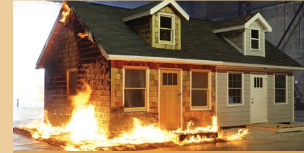
COMPARISON of combustible, cedar-shingle siding product (left) vs. fire-resistant, fiber-cement siding when exposed to a simulated ember storm.
