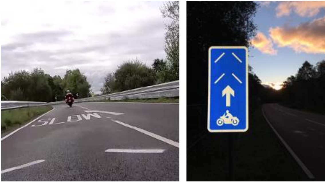
Figure 1: PRIMES 'gateway' design PRIME road marking (left) and PRIME road sign (right)
