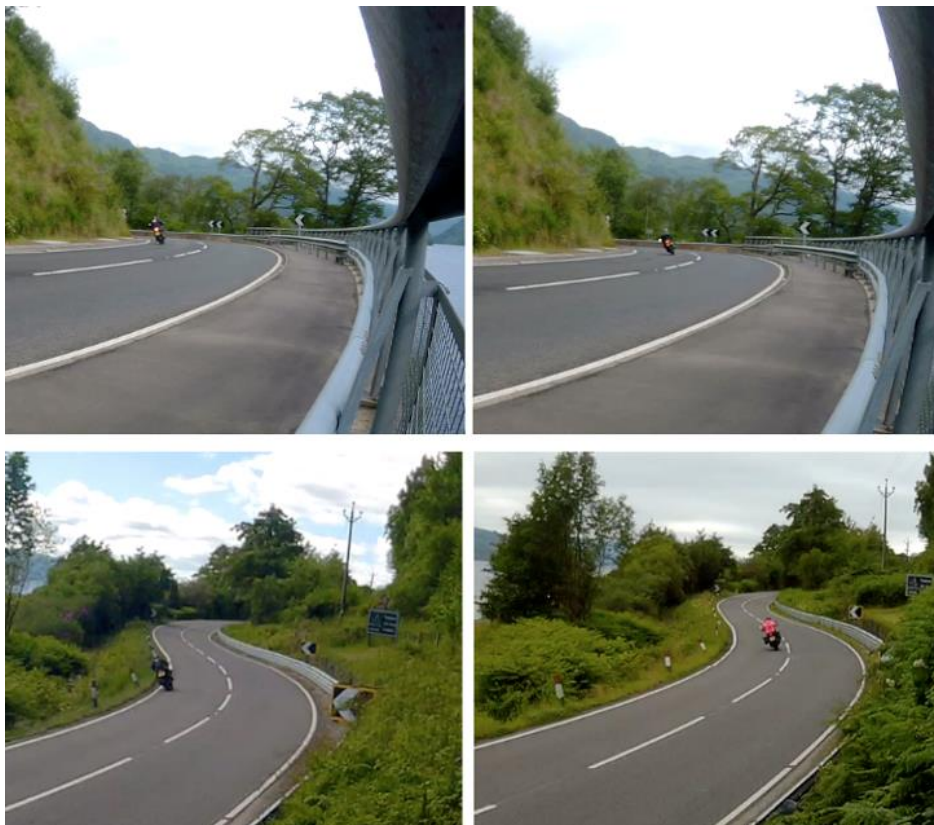
Figure 9: Changes in road position (left-hand images = without PRIMEs installed, right-hand images = with PRIMEs installed)
