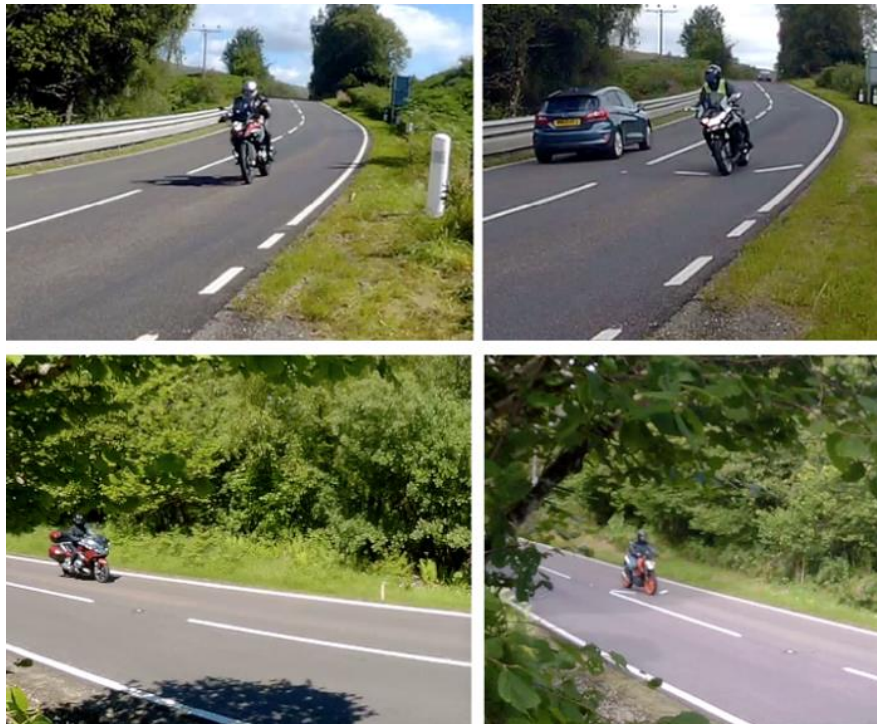
Figure 8: Changes in road position (left-hand images = without PRIMEs installed, right-hand images = with PRIMEs installed)
