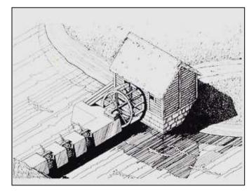
16 feet in diameter. The millstones were cut from native granite located on the east side of Lake Winnipeg. These massive stones measured five feet in diameter, were eight inches thick and had to be transported by York Boat to the site of the mill.
