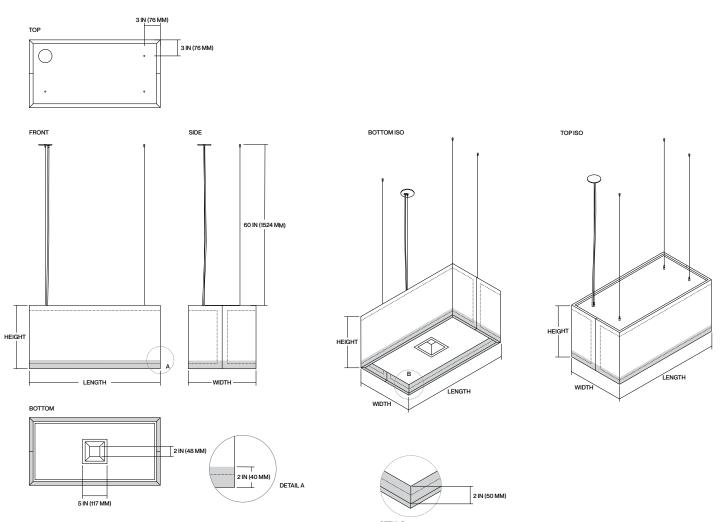
DETAIL B LIGHT PANEL REGRESSED INTO FIXTURE
