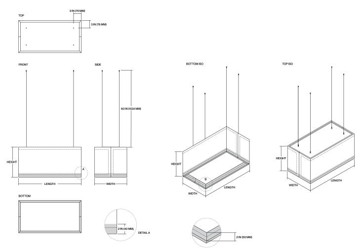
DETAIL B FELT PANEL REGRESSED INTO FIXTURE
