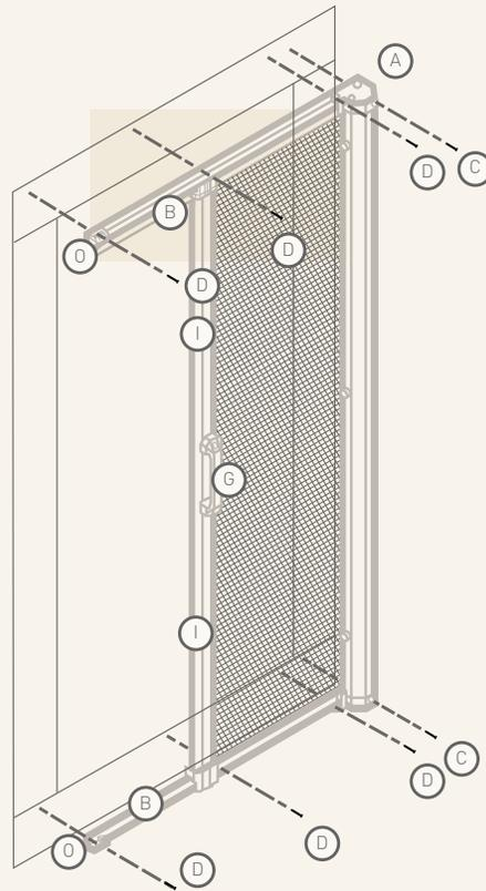
**Detail of track position in relation to the housing and housing end cap**
