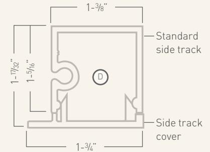
Cross sectional view of the standard slidebar and 4" bottom seal
