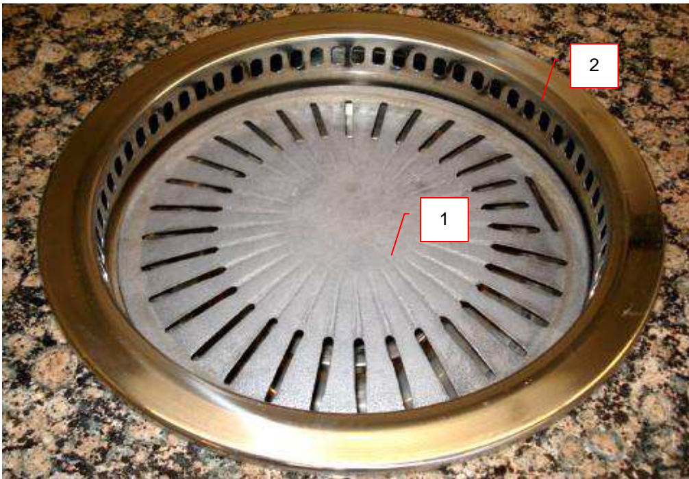
Photo 2 - Grill Surrounded by the Vented Top Cover
