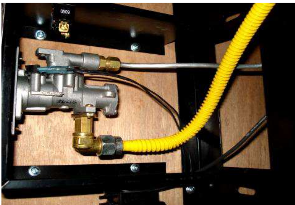
Photo 4 - Gas Control Valve manufactured by Sangium Micron (V-037C)
