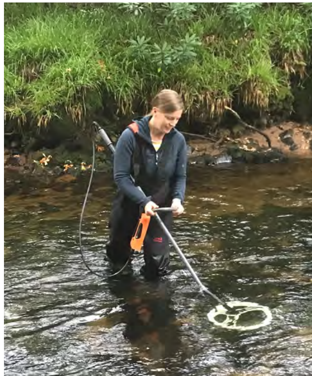
Figure 6: Scanning the river bed for hidden mussels using a Biomark antenna and reader.
