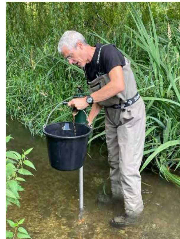
Figure 1: Sampling the hyporheic zone using a Bou Rouge sampler. Photo by Judy England.
