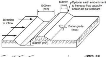
1. Diversion drain. The drain channel must be at least 150 mm deep with a curved shape that will be site specific. Stabilise the flow path to protect it from scour by lining the drain with matting or rock. If dispersive soils are present, create diversion drains by building soil berms instead of digging.
