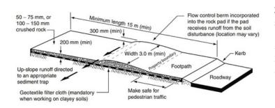
3. Stabilised site access. Stabilised access is from the site boundary to a formal stockpile area or work site; minimum length for small developments is 10 m. Strip at least 150 mm of topsoil, cover with geotextile then a 200 mm thick pad. Divert water from this control to appropriate sediment controls.
