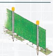
5. PROTECT STORMWATER CONNECTION PIT (pg. 61) This is your last line of defence against sediment escaping. Protect the stormwater system from blockage and accumulation of sediment / building debris using sediment fences / mulch bunds, filter socks and stormwater pit traps.
