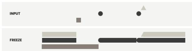
At any time you can hold the footswitch to lock in the current sound, so you can play freely overtop without replacing it.
