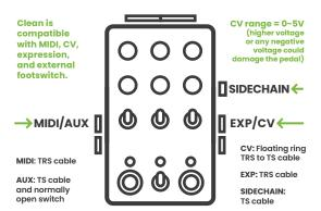
CV and expression can be used to control Clean's knobs.
