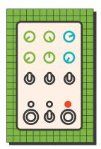
Clean's limiter is actually a clipping circuit with a wide range, variable threshold. This means you can set the threshold so low that it starts to rip into your sound and distort it, and that's what Dusty mode lets you do. SENSITIVITY sets that threshold and works loosely as an "amount" control.
