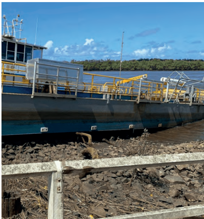
Figure 12: The Burns Point Ferry, stranded after its submarine cable snapped during the flood. Note the chain mooring the ferry to the piling on shore in the foreground, which prevented the total loss of the vessel. (Photo courtesy of Risk Frontiers 2022)
