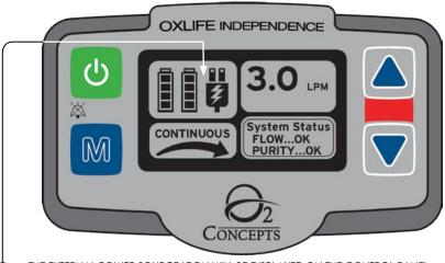
THE EXTERNAL POWER SOURCE ICON WILL BE DISPLAYED ON THE CONTROL PANEL.
