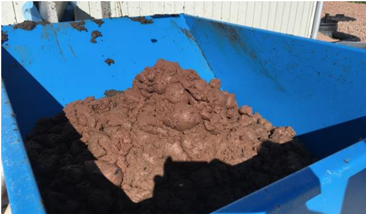
Figure 3. Picture of wet fish sludge with TSS of about 20 %, produced from Fifax RAS.
