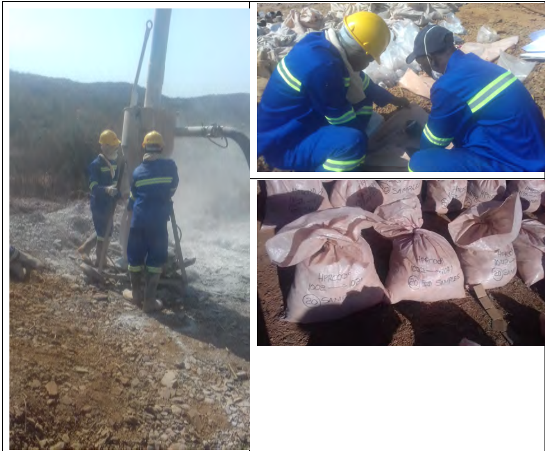
Photo 8: Sampling at the Rig, Packing and Labelling Samples
