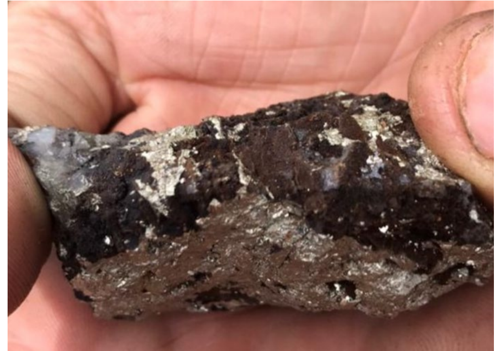
An example of heavily pyritized quartz from the Golden Valley Project area, an indicator of potential for gold mineralisation
