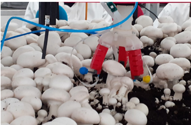
Figure 6. Gathering data on the forces required to harvest a mushroom (top) and prototype of a soft gripper for harvesting mushrooms robotically (bottom). - Photos by H. Grogan
